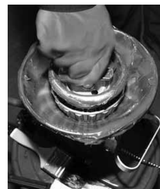
Fig. 22. Mechanical grease packer.
