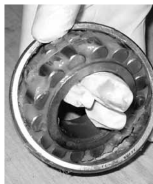
Fig. 21. Grease can easily be packed by hand.
